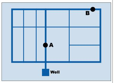
Looped distribution systems such as this one allow water to flow freely in all directions. In this system, only two sampling locations are necessary to provide samples representative of the main loop (**A**) and the branch loop (**B**) conditions. (Adapted from *A Guide to Bacteriological Sampling of Public Water Supplies,* Virginia Department of Health, January 7, 1998.)
